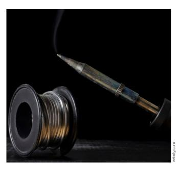
Flux Cored Solder Wire (Quality Control) Order, 2023 includes a specific type of solder wire that has flux in the centre of the wire. Without flux, wire solder would be difficult to use. It is used in soldering electronic components, automobiles, telecommunication and diverse engineering industries.
